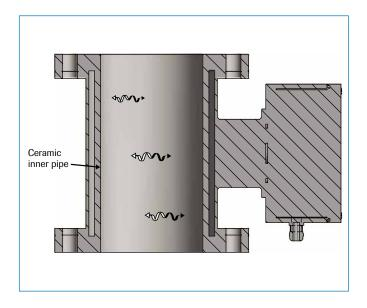
With the design in DN 70 mm, the connection flange could be freely selected.
